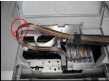
The tube is excessive long.
